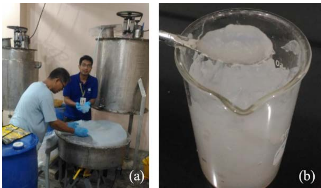
Figure 3. Large scale production of the NC-TEMPO (a) showing the 500-liter fermentor and collecting the CNF-TEMPO; (b) gel-like CNF-TEMPO slurry. (With permission to use photos from the authors.)
